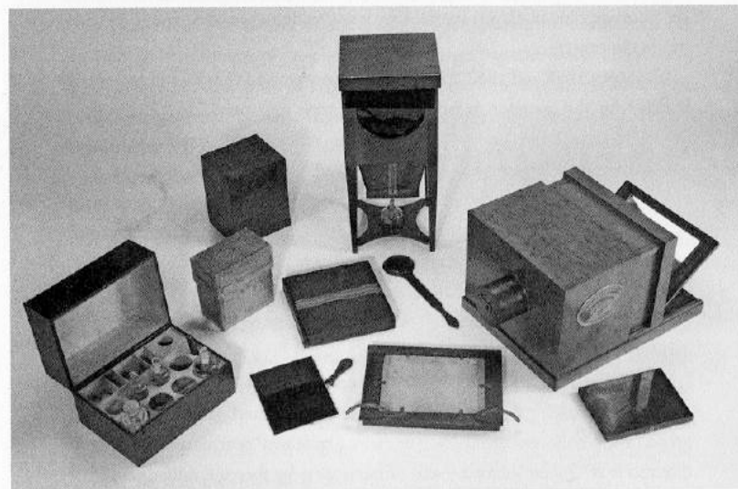
Figure 41. Giroux daguerreotype camera, 1839. Courtesy of the George Eastman House, International Museum of Photography and Film.
